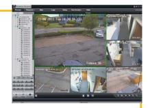
duplex display and recording capabilities. The recorders are able to record real- time at 2CIF resolution and offer selectable CIF, 2CIF and 4CIF record resolution.
